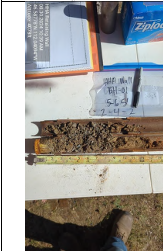
Picture # 3: BH-01 SPT 5-6.5 ft
